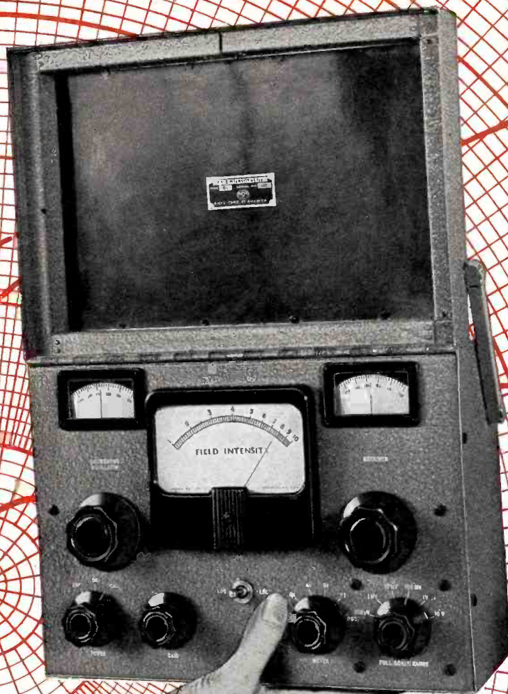
The new Portable Field-Intensity Meter, RCA Type WX-2B shown one-third actual size. A loop antenna is built right into the lid!
